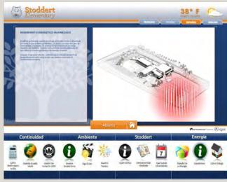
Stoddert is the first school in Washington, DC to use a ground source heat pump system (aka "geothermal") to heat and cool the entire building. 72 wells were drilled below the sports field (as displayed on the green screen).
