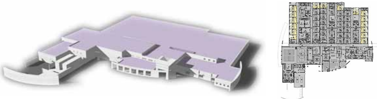
Previous prototype elementary school floorplan. Only 15 out of 42 classrooms had windows for views, not daylighting
