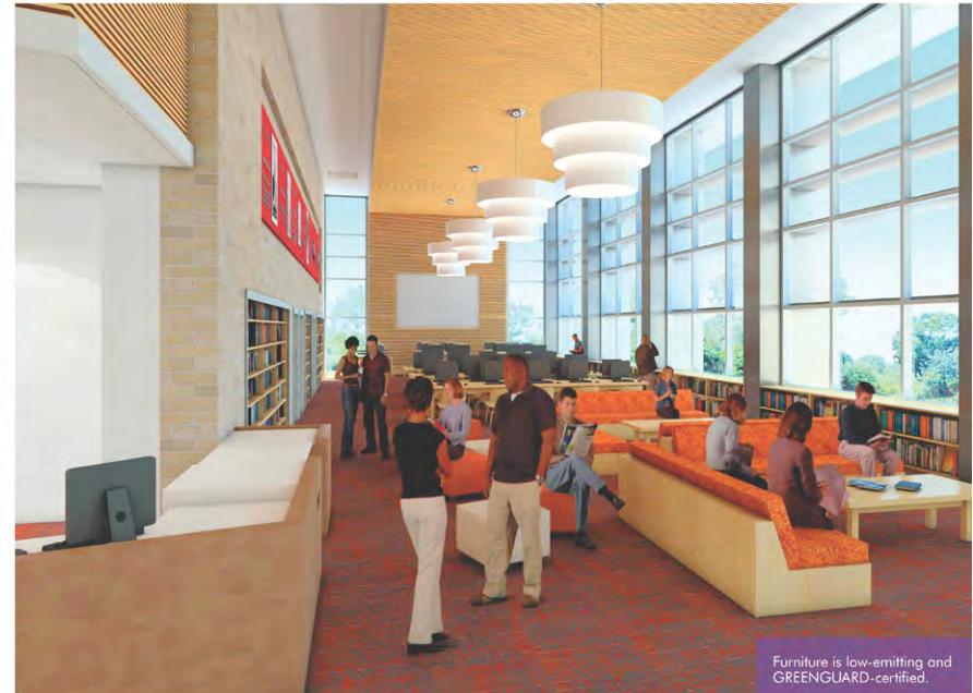
Full-height walls, absorbent ceiling assemblies, and strategic placement of HVAC equipment improve the acoustics of the classroom.
