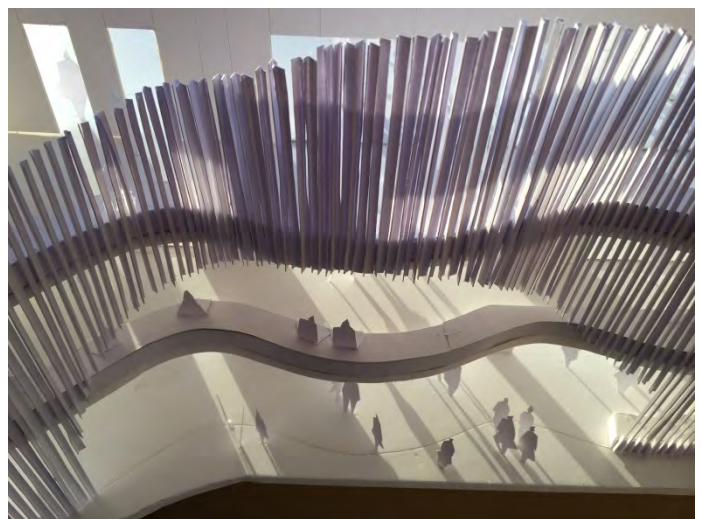
Physical model of Cruci testing the play of natural light and sculpted welcoming entry form. The physical model was a critical design communication tool greatly assisting stakeholder engagement.
