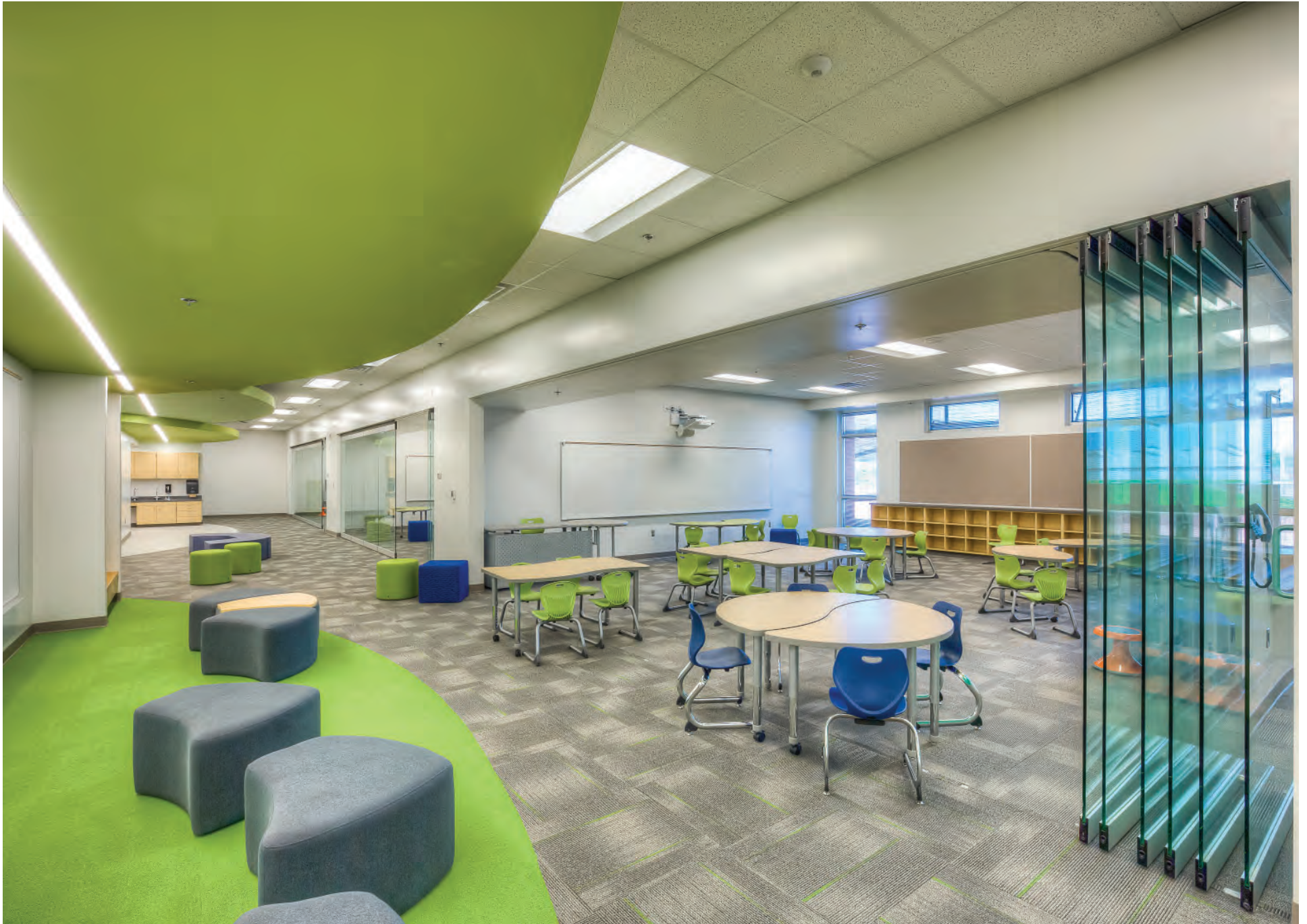
Operable glass walls provide varying degrees of openness. Comfortable and flexible furnishings are used throughout. Storage space is minimal, provided for only in the millwork and furniture, a decision resulting from a great deal of discussion during design.
