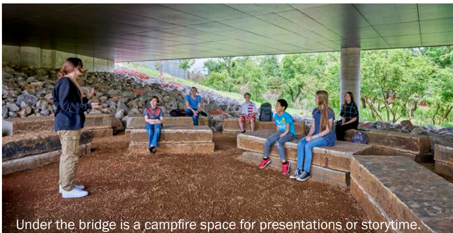
Boulders found on the site were re-purposed as retaining walls.
